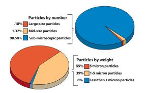
This could be expressed as an 80% removal rate – by weight. But, as these charts show, particles larger than 5 microns account for only 0.18% of the total number of particles in the air. That 80% figure sounds impressive, but it still leaves 99.82% of the particles still circulating!
